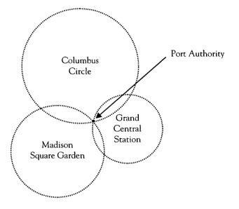
This process of calculating a single location using multiple linear measures is known as trilateration.<sup>34</sup> GPS receivers use trilateration in three dimensions (based upon information received from four satellites) to calculate their latitude, longitude, and altitude.<sup>35</sup> In addition, a receiver can compute its speed and the direction in which it is traveling by assessing the rate of change in information received from the satellites.<sup>36</sup>
